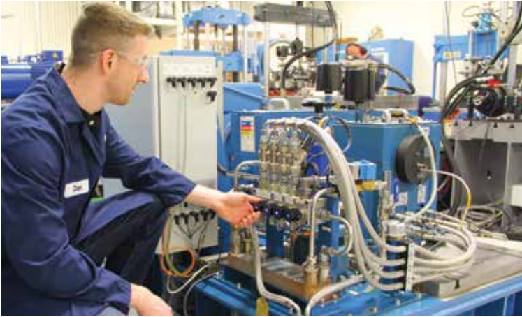
NPDC product engineer calibrates one of the new rolling element test rigs.
